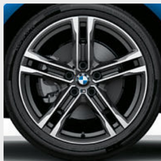
■ 18" M light alloy wheels Double-spoke style 819 M Bicolour Orbit Grey metallic, gloss-lathed, wheel size 8J x 18 with 225/40 R18 tyres. 5
